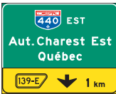
Advance exit sign
